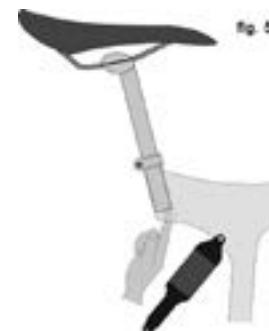
**WARNING:** If your seat post is not inserted in the seat tube as described in B.1 above, the seat post, binder or even frame may break, which could cause you to lose control and fall.
